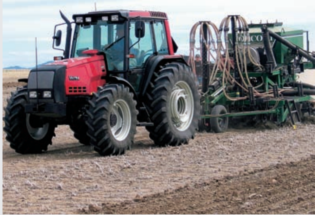
The Valtra 6800 plays a key role in NARC's evaluation of air drill-based seed and fertilizer placement systems with two different research-scale air till drills.
